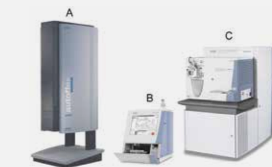
Proteomic equipment available at ZBS 6. A: AutoFlex Speed MALDI-TOF mass spectrometer (Bruker Daltonics). B: EASY-nLC Liquid Chromatograph (Thermo Scientific). C: LTQ Orbitrap ESI mass spectrometer (Thermo)
